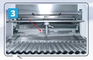
The Adjustable Variable Speed Diverter Bar Above the Product Channels, Sweeps **Back** & **Forth** to Eliminate **"Twinning"**
