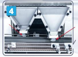
Flexible Silicone Funnels Finish the Process by Reducing the Incidence of **Gummies** Clogging the Funnels
